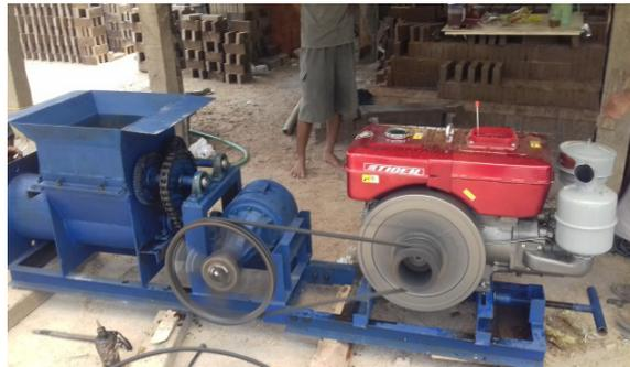
**Gambar 2. Mesin Batu Bata Press Kapasitas 1000 pcs/jam**
